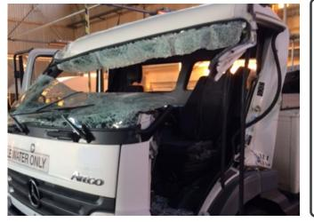
A water truck had to get out of the way due to oncoming traffic. The truck hit the RH wing of the aircraft.
